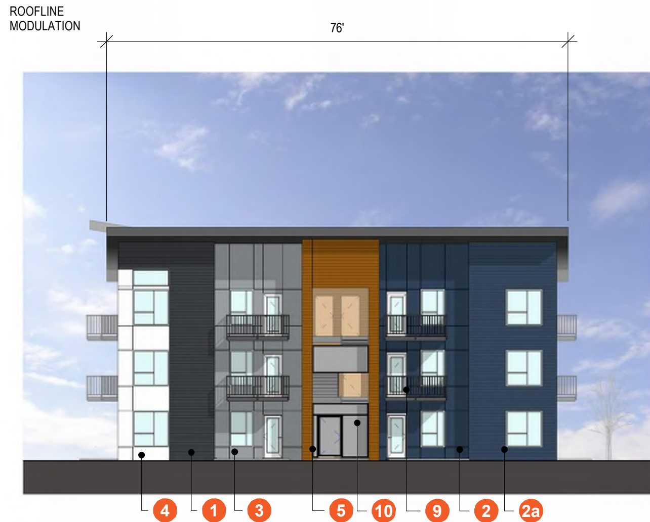
② ELEVATION: PERIMETER BUILDINGS (CEFH) - PARKING SIDE 1/16" = 1'-0"
