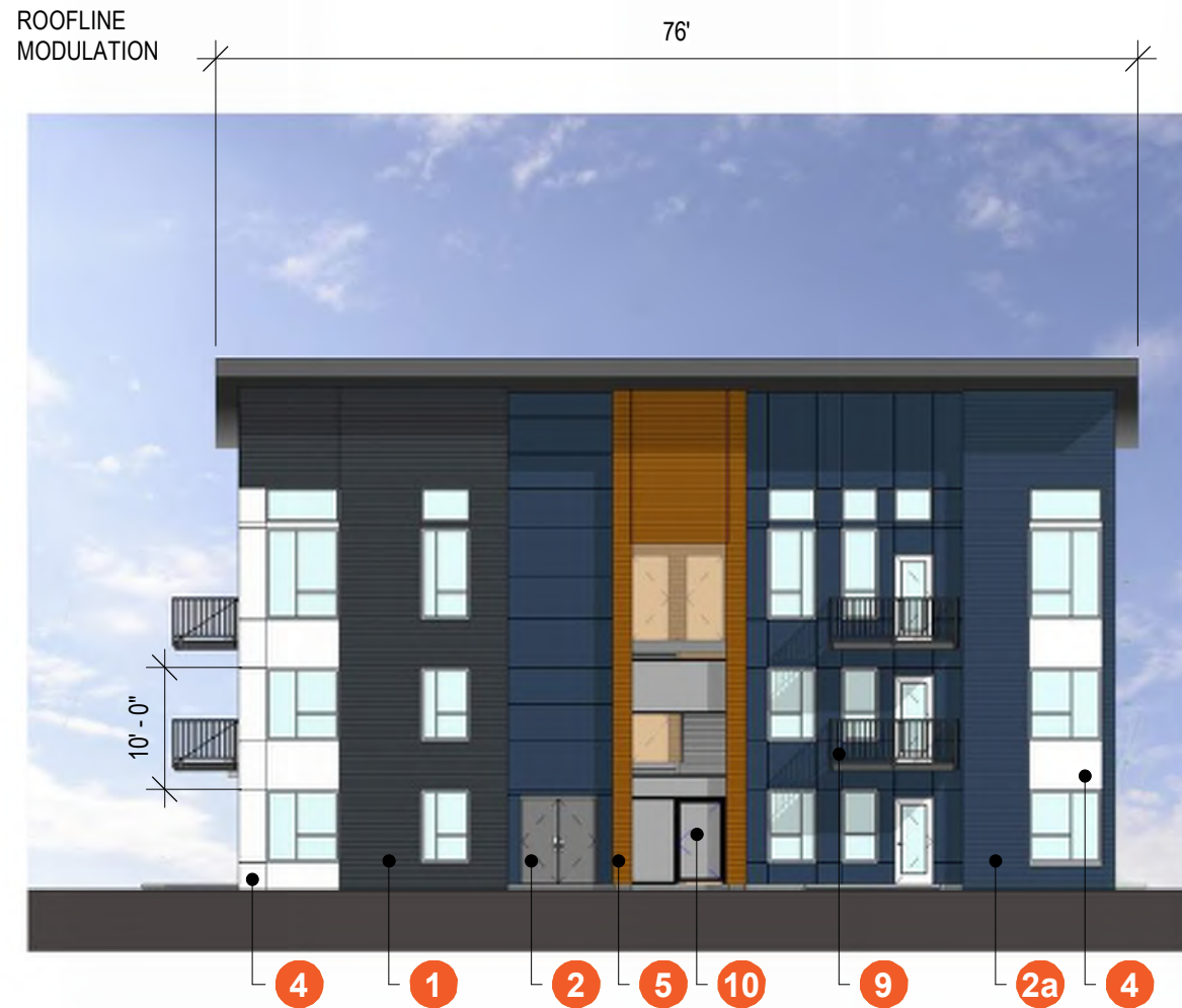
② ELEVATION: CITY BUILDINGS (A&B) - WOONERF SIDE 1/16" = 1'-0"
