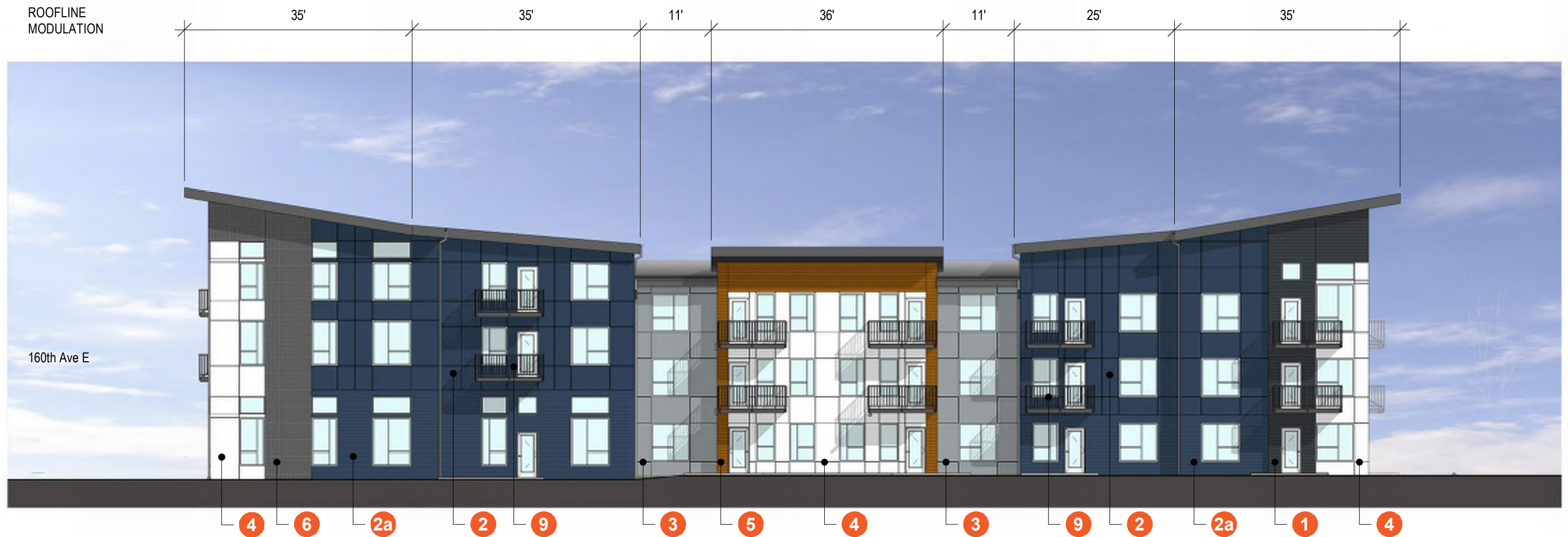
① ELEVATION: CITY BUILDINGS (A&B) - PARKING SIDE 1/16" = 1'-0"
