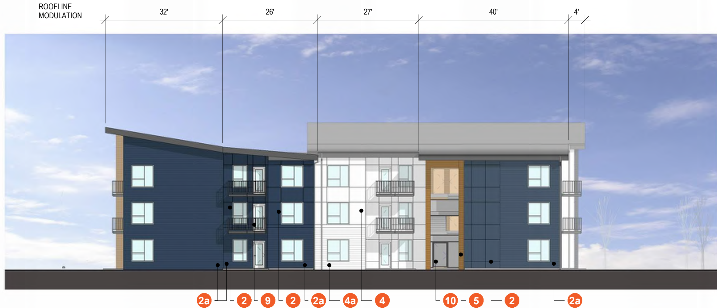
① ELEVATION: PERIMETER BUILDINGS (CEFH) - COURTYARD SIDE 1/16" = 1'-0"
