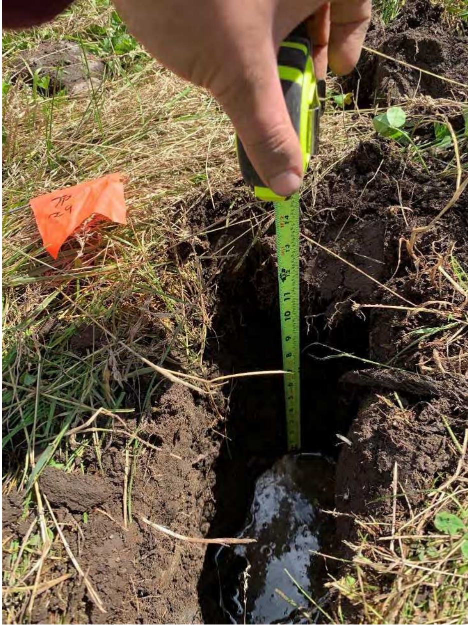
7-Measurement of Water Table at 12 Inch Depth at TP29 (Taken 6/17/20)
