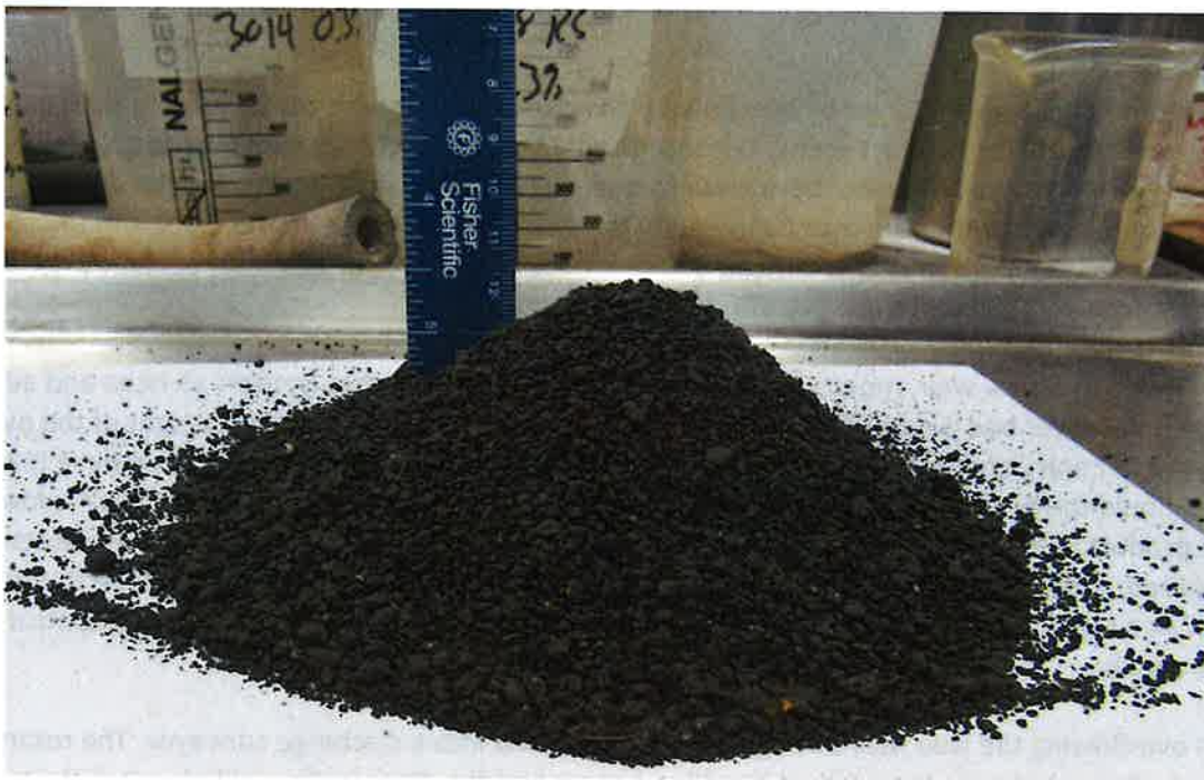
Dried Product from Pilot Testing Sumner, WA Biosolids - K-S Lab Test TPG-8907
