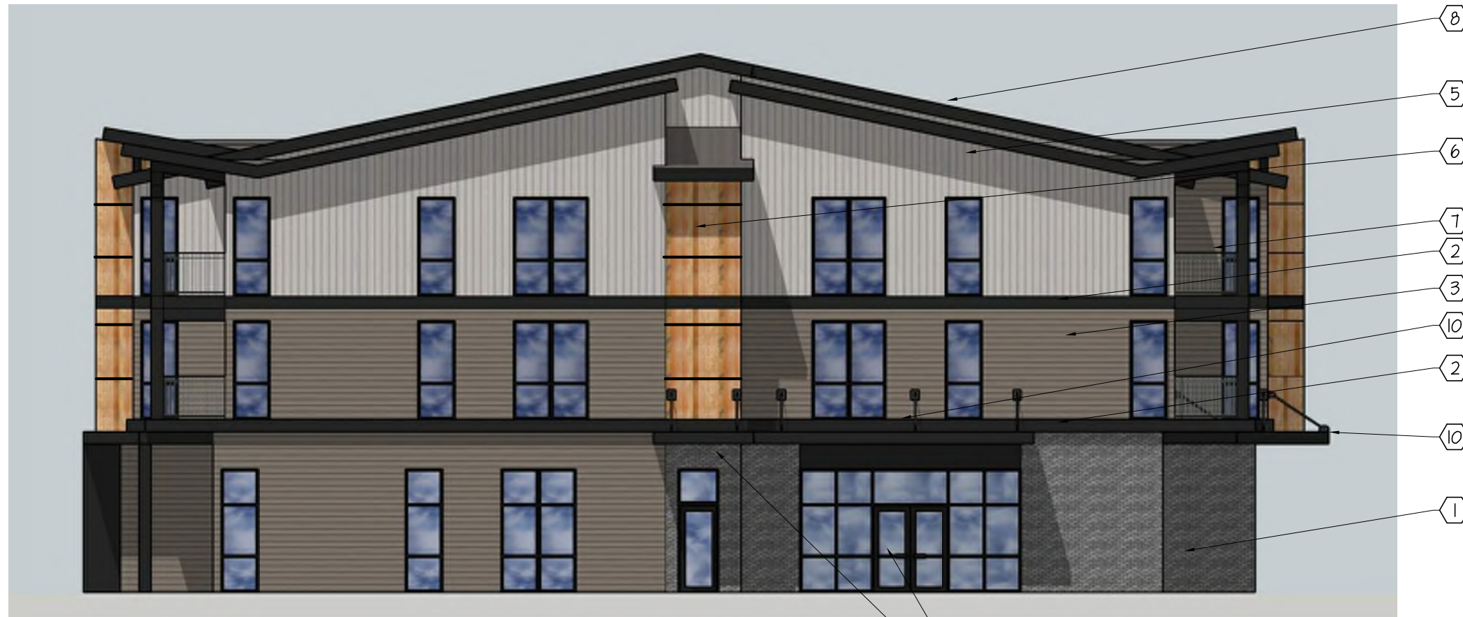
3 BUILDING 1 EAST ELEVATION - EAST OPP. SCALE: 3/32" = 1'-0"
