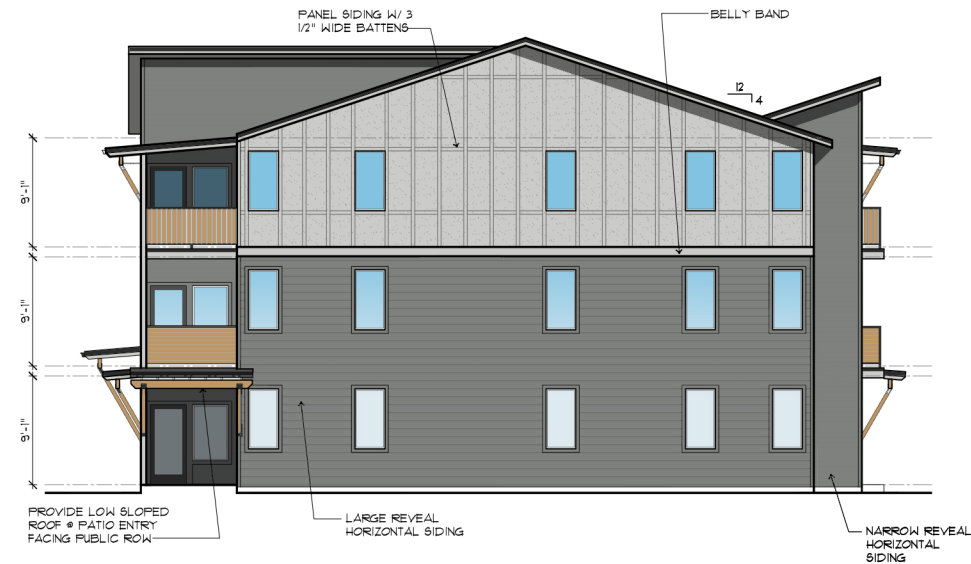
Buildings 2 - Side Elevation (Building 3 Mirrored)
