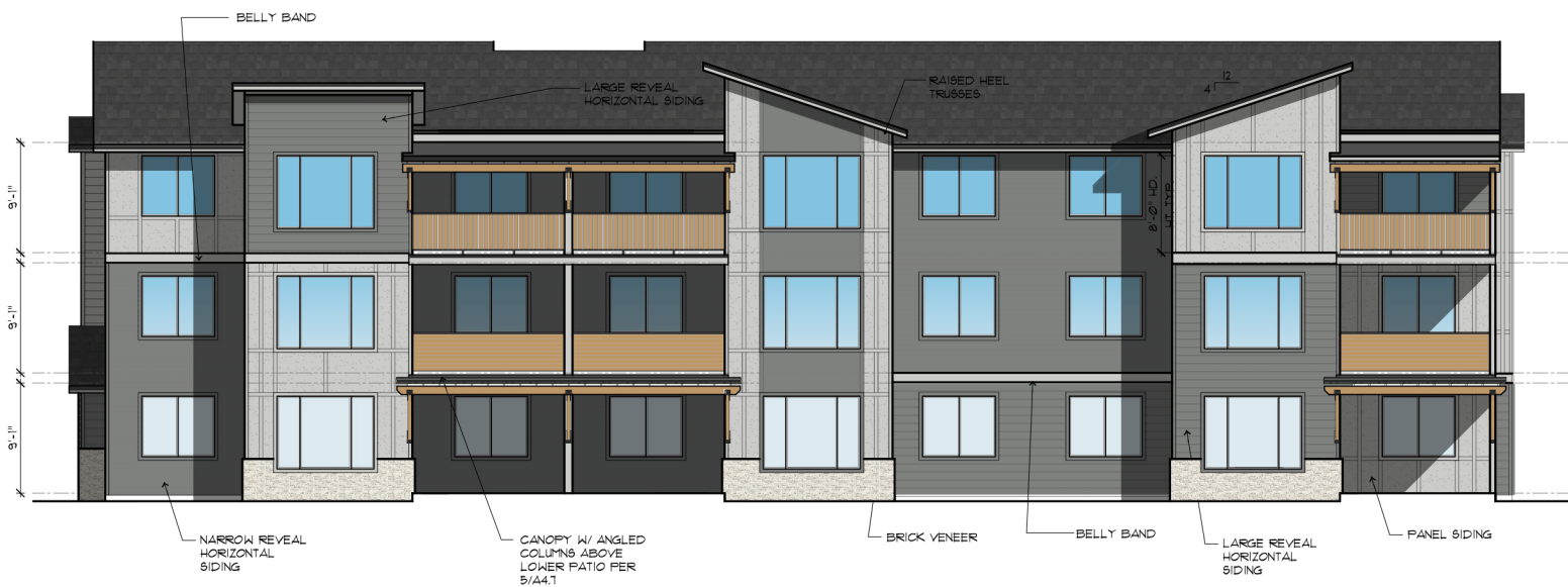
Buildings 2 - Rear Elevation (Building 3 Mirrored)
