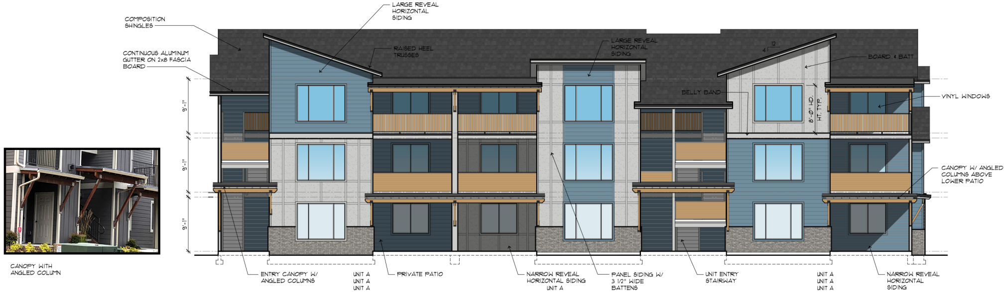
Buildings 1 & 5 - Front Elevation (Building 4 Mirrored)
