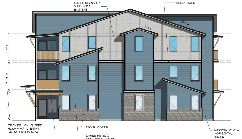
Buildings 1 & 5 - Side Elevation (Building 4 Mirrored)
