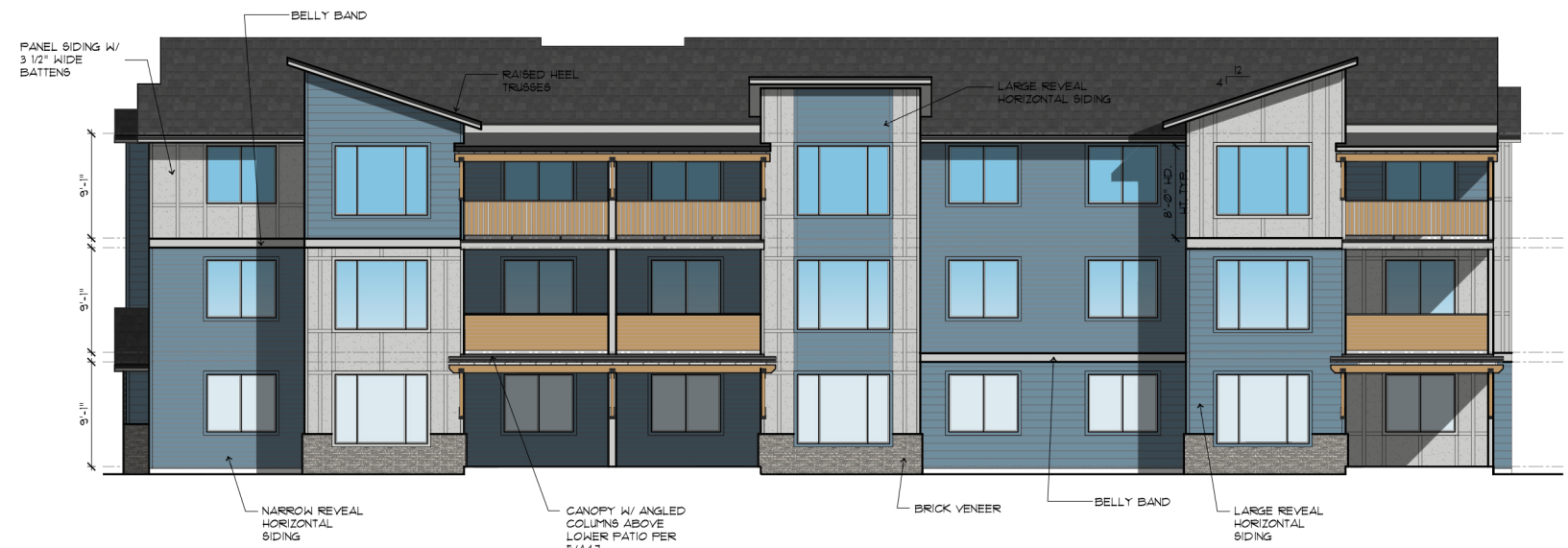
Buildings 1 & 5 - Rear Elevation (Building 4 Mirrored)
