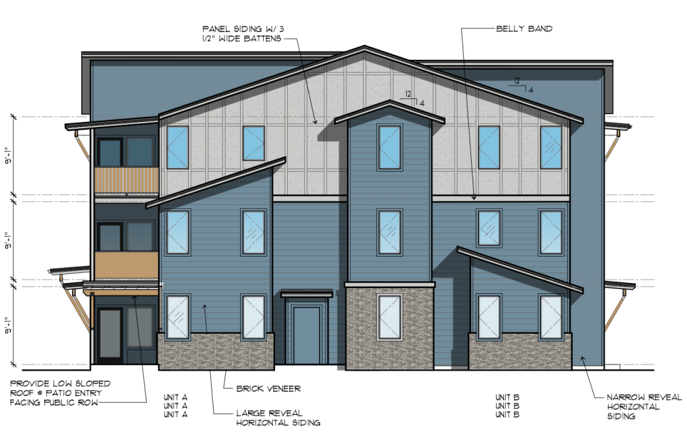
Building 7 - Side Elevation SCALE: 1/8"=1'-0"
