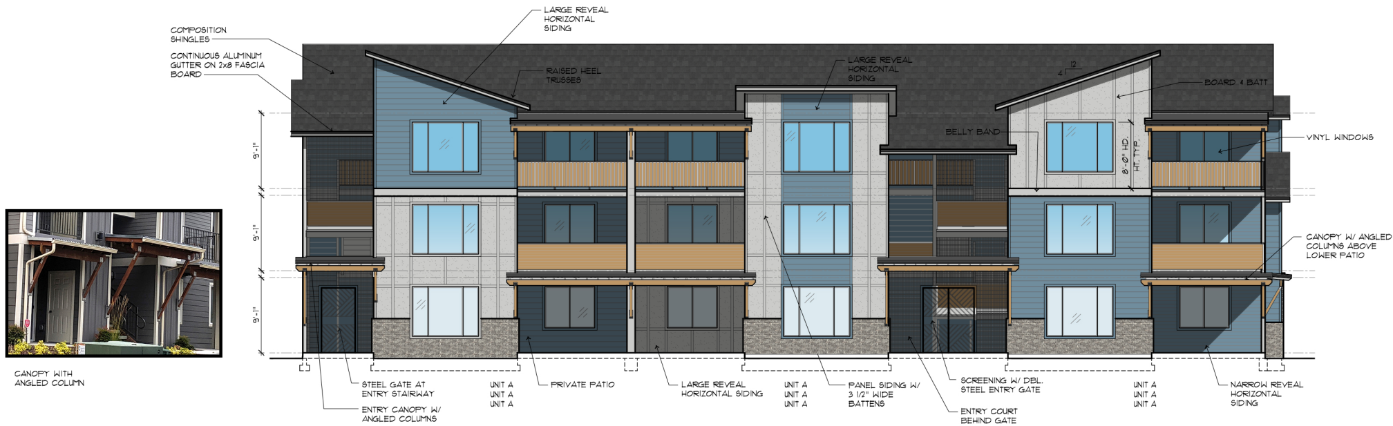
Building 7 - Front Elevation SCALE: 1/8"=1'-0"
