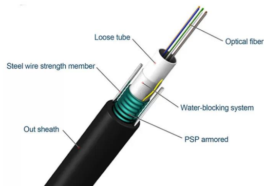
Figure 14 - Loose Tube Aerial Cable
