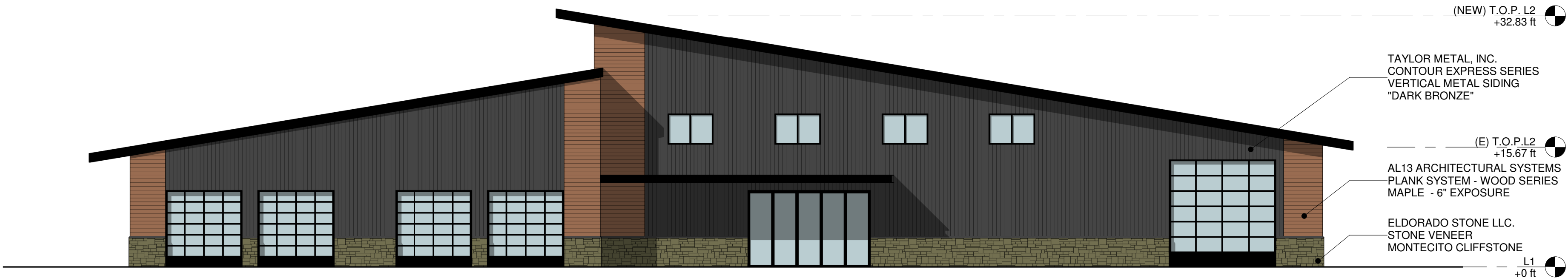
EXTERIOR ELEVATION - SOUTH - 160TH STREET
