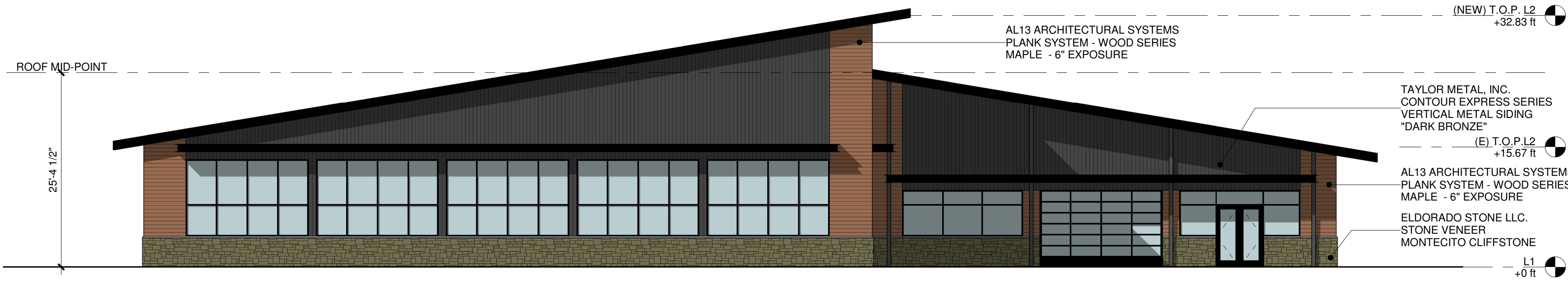
EXTERIOR ELEVATION - NORTH - 60TH STREET
